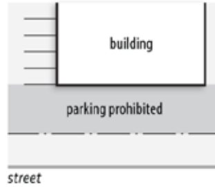
Figure 20-5: Parking Prohibited between Building and Street Right-of-Way
