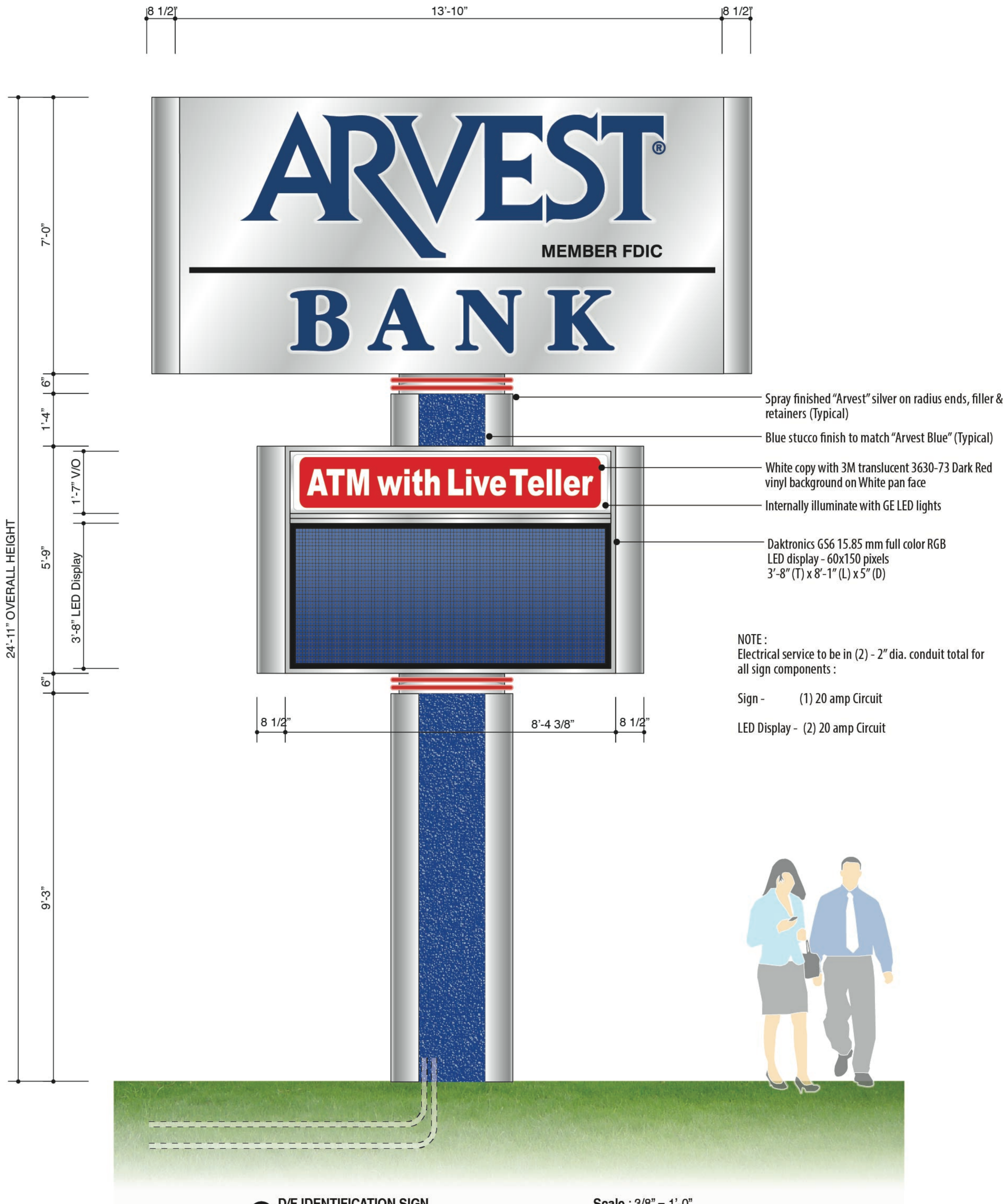
1 D/F IDENTIFICATION SIGN Scale : 3/8" = 1'-0" -Manufacture shorter pole cover by 8" to allow room for larger LED display -Remove existing Marquee sign & install new Daktronics LED display
