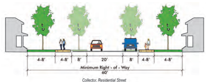
Figure 17: Sample Residential Collector Street Cross Section
