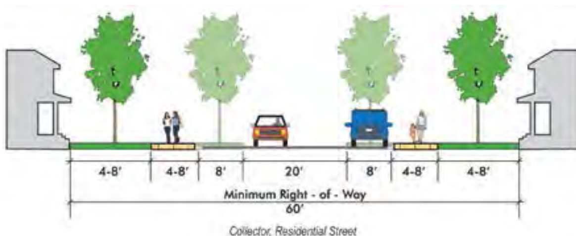
Figure 8: Sample Residential Collector Street Cross Section
