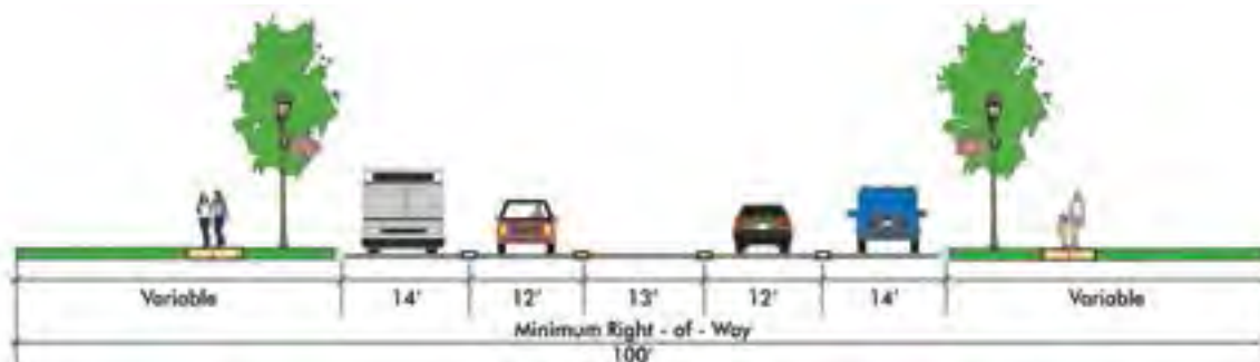
Figure 7: Sample Commuter Street Cross Section
