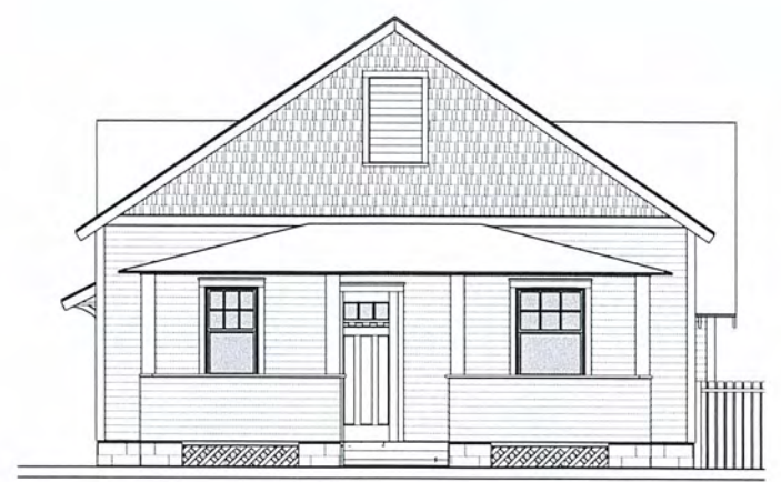
③ East Overall Building Elevation 1" = 10'-0"
