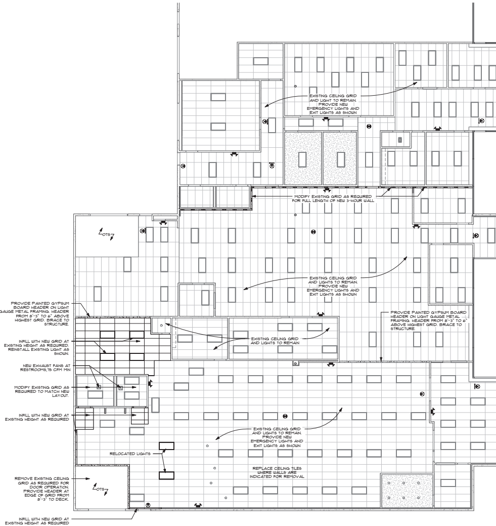
A FIRST FLOOR REFLECTED CEILING PLAN 1/8" = 1'-0"
