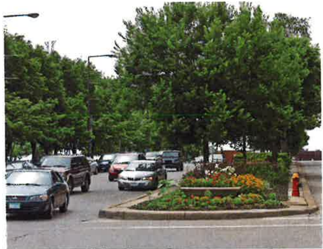
Medians can provide space for street trees, gateway treatments (such as planters) and utilities (such as fire hydrants.)
