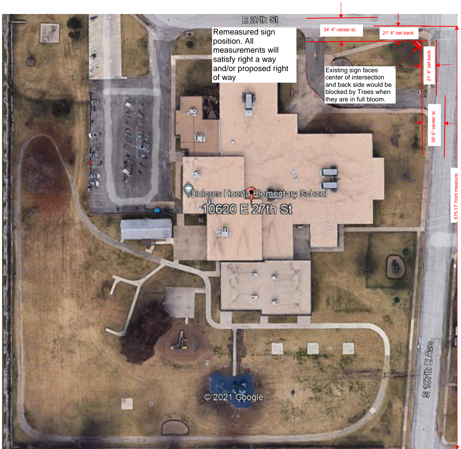
Revised overhead Site plan showing corrected measurements to satisfy Right-of-Way and/or Planned Right-of-Way requirements
