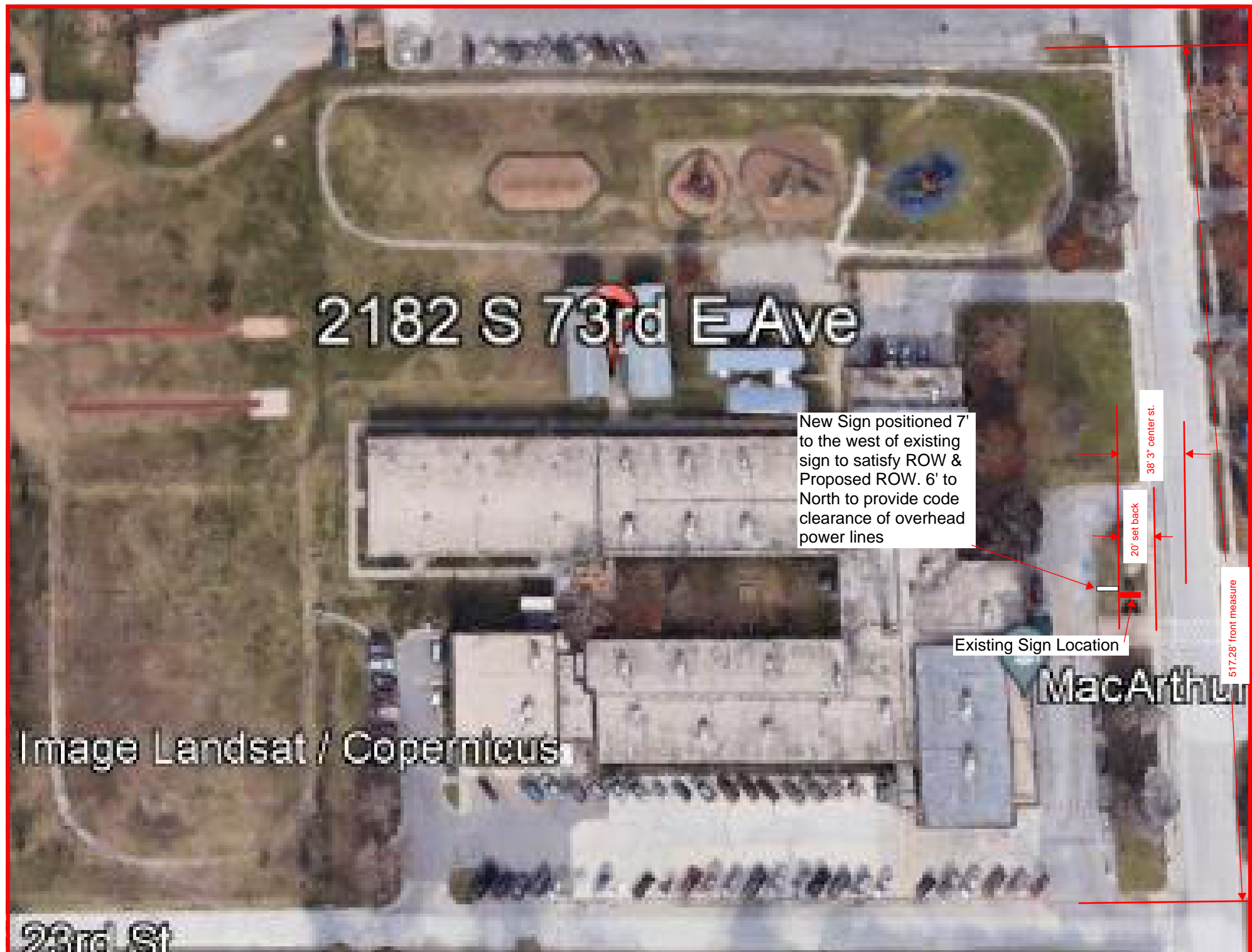
Revised Overhead plan showing repositioning of sign to satisfy Right of Way requirements
